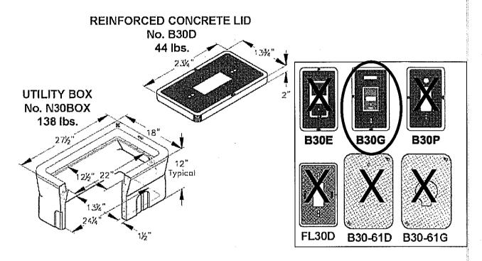
A high density reinforced concrete box with non-pettling shoulders positioned to mointain grade and facilitate back filling. Appreximate dimensions and weight shown.
